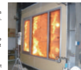
Combustion test to evaluate fireproof performance
