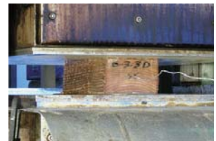
b) 圧縮開始 b) Start of pressing, deforming in the thickness direction.
