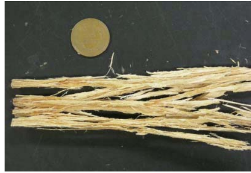
第7図 常温圧縮変形時の繊維束の例 Fig. 7. Fiber bundle of deformed wood compressed without heating.
