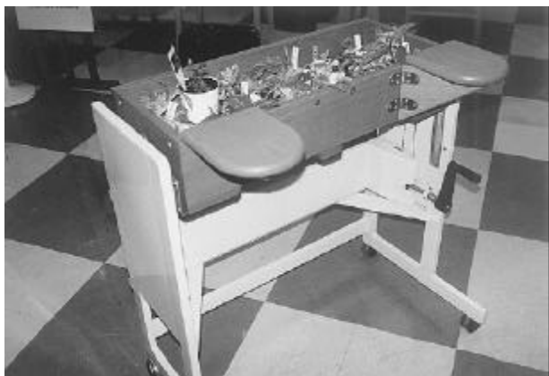
第7図 屋内用木製移動式花壇(昇降タイプ) Fig. 7. Wooden portable flower bed for the indoor (the going up and down type).
