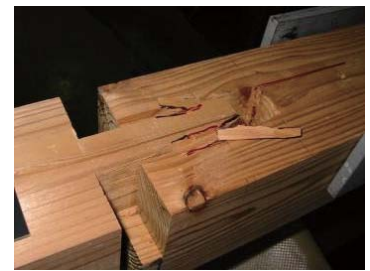
第7図 鎌の圧縮破壊 Fig. 7. Compression failure of kama-ago ( koshikakekama-tsugi joint).
