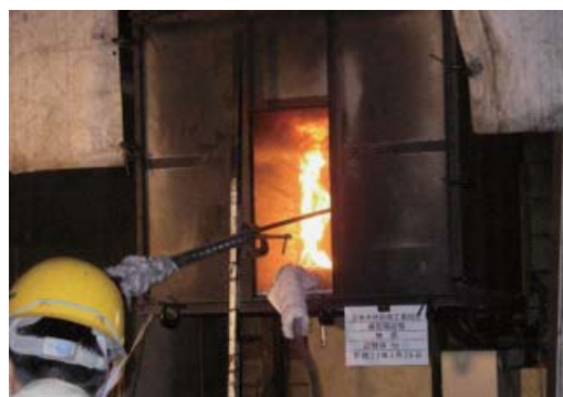
第 12 図 加熱中の供試箱の状態 (処理材 B) Fig. 12. Appearance of test-box during heating (treated sample B).
