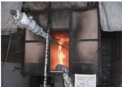
第 9 図 加熱終了時の供試箱の状態 (処理材 A) Fig. 9. Appearance of test-box after heating (treated sample A).
