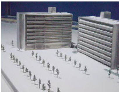
As a result of snow wind tunnel and other tests, we have suggested a shape and layout for buildings to help prevent snow cornices, snow accretion and drifts, reflecting them in the design of buildings.
