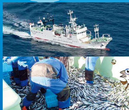
The third Hokushin-maru scientific research vessel was completed in November 2014. Using the cutting-edge devices (a pelagic and/or mid water trawl net, multipath ultrasonic flowmeter, etc.) in this vessel, surveys are conducted on the distribution densities of Pacific saury and other migrating fish, water temperature and flow, and the results are released as migrating fish news. Such information is used to increase the operational efficiency of fishery operators and marine product companies.
