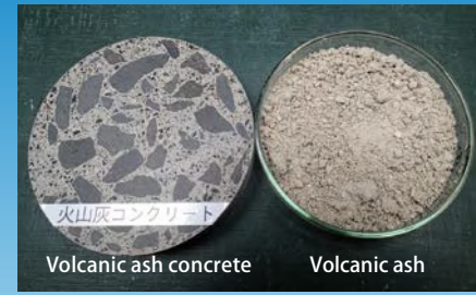
We have developed the method to product long-life concrete using volcanic ash in Hokkaido.
