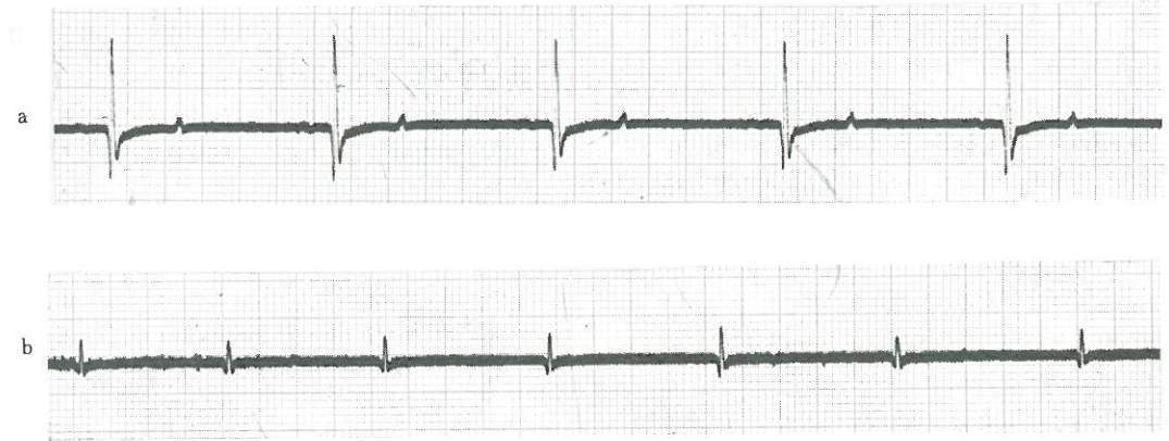
Fig. 4 Recording of ECG-signals from an adult Holstein cow by radio telemetry using an improved transmitter (a) compared with early one (b).
