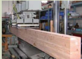
Bending strength test of full-size timber
