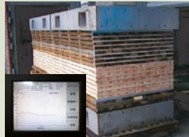
Automatic control system of artificial drying equipment
