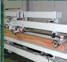
Correction Cutter Machine For molder datum level
