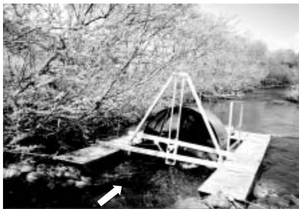
Fig. 23 A rotary-screw trap operated in the Masuhoro River, Hokkaido. The arrow indicates flow direction.
