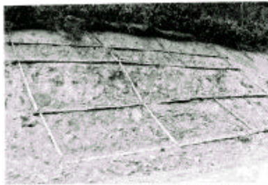
写真-10 植栽直後の実験林 No.2 植栽試験地と面状基礎工 Photo. 10. Expt. For. No.2 planting test plot, immediately after planting.
