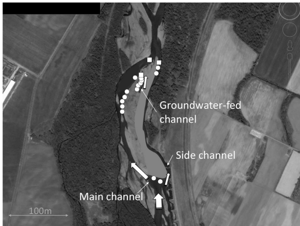
Fig.3 Locations of piezometers installed for evaluating vertical hydraulic gradient (open circle) and of fish populations surveyed (open square) in each channel type. Arrows indicate flow direction.
