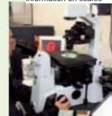
Identifying a label on the otolith by inverted microscope
