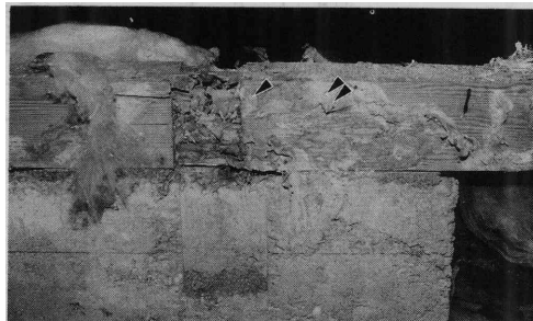
写真39 CCA加圧注入土台上の菌系生長 (▲) と腐朽状況、中央のほぞ穴付近 (▲) Photo.39. Hyphal growth (▲) on the surface and decay beside the tenon (▲) of the CCA-treated sill.
