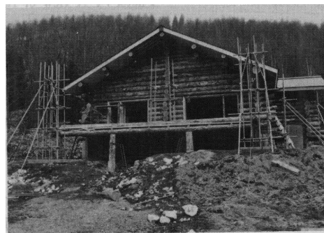
写真13 X方向加力の全景 Photo . 13 . A view of racking test (X - direction)
