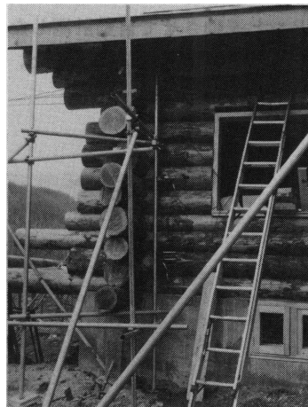
写真11 建物Bの交点 ( X_5 Y_1 ) の変位計 (X方向加力) Photo . 11 . Displacement instruments at intersection ( X_5 Y_1 ) of Build B (X - direction)
