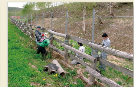
Technology for estimating durable life of wooden buildings Technology is developed for estimating degraded state and durable life of existing buildings in order to properly maintain and control wooden road guards.
