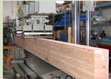
Bending strength test of full-size timber
