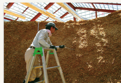
Wood fuel quality control technology Research is performed at the chip-drying facility utilizing natural energy to optimize the quality control technology needed for efficient use of wood fuel.
