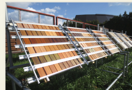
Technology to improve weather resistance of painted materials To lengthen the durable life of exterior products, wood surface treatment technology is developed to improve weather resistance of painted materials.
