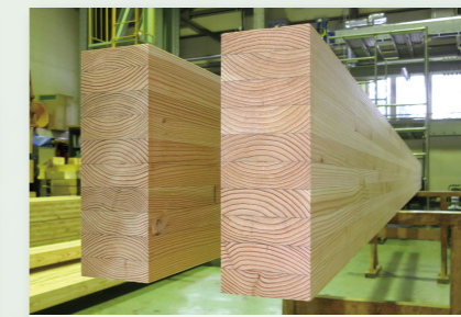
High-strength Japanese larch laminated materials Research is being made for developing high-strength laminated materials for buildings (laminated timber, LVL) that feature strength properties of medium-large-diameter larch timber.
