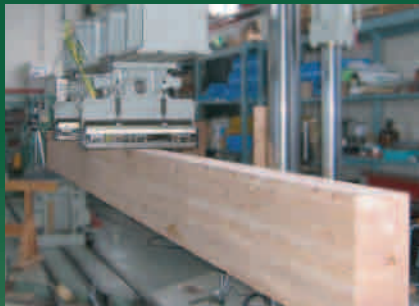
Flexural strength tests of actual-size material
