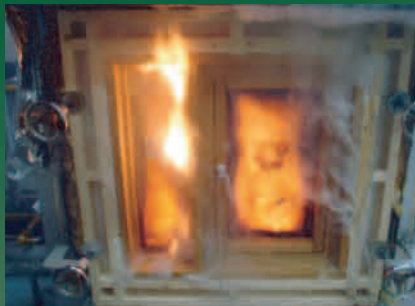
Fire protecting test on wooden sash
