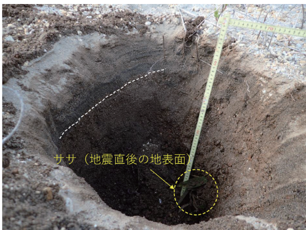
写真7 3月の崩壊堆積物の本体(白破線より下位)と後続の流水による堆積物(白破線より上位) Photo 7 The main body of the landslide sediment in March (below the white dashed line) and the subsequent sediment due to running water (above the white dashed line)
