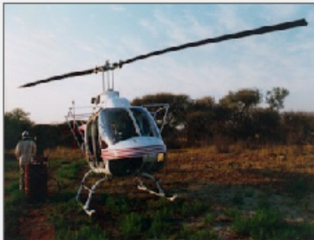
Survey helicopter with distance interval markings fixed to external cage. Used for large mammal surveys, Madikwe Game Reserve, South Africa Photo: K...
