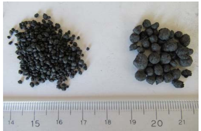
写真2 ガス化副産物造粒物の一例 Picture 2. Granulated samples of gasification biochar
