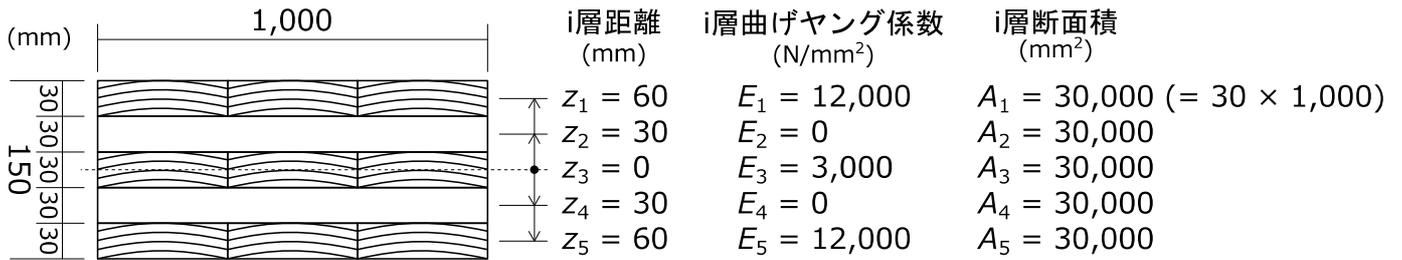
$$I_i(i=1\sim5) = 1,000 \times 30^3 / 12 = 2,250,000 \text{ mm}^4$$
